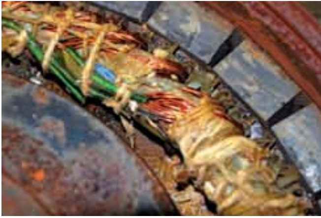
An insulation failure in these high-voltage windings led to arcing between wires.
